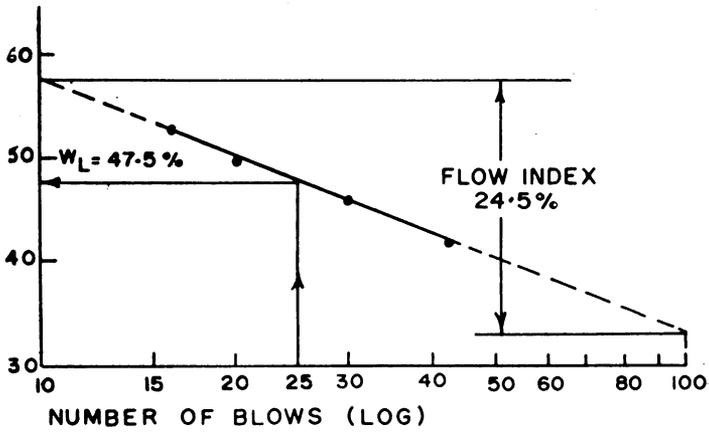
Fig. 4.3 Flow curve for liquid limit determination
