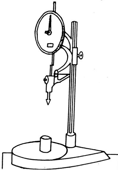
Fig. 4.4 Cone penetrometer for limit determination
