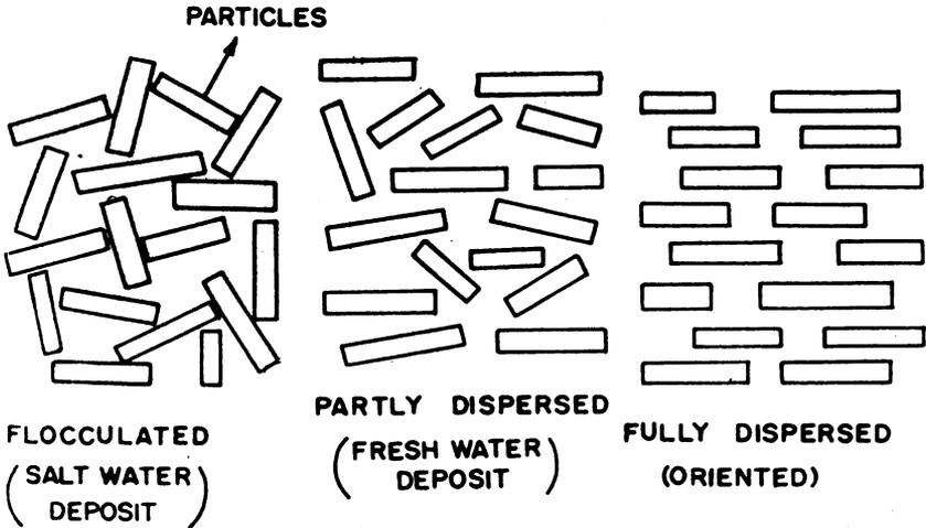
Fig. 2.5 Basic clay structures. Structures of salt water and fresh water clay deposits
