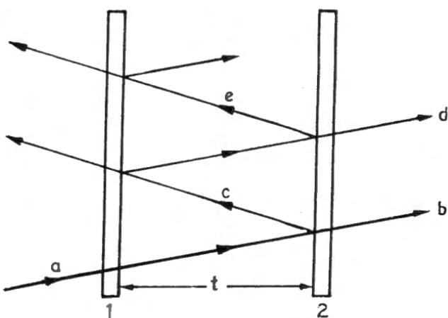
Fig. 3.5 : Schematic diagram of a Fabry-Perot interference filter. For clarity, the distance between the two plates is shown excessively large. Normally,  $t$  is of the order of few  $\mu\text{m}$ .
